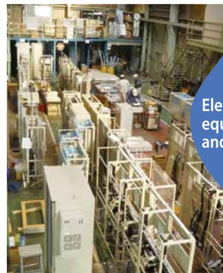
Inside the electrical equipment factory. Various control panels being manufactured
