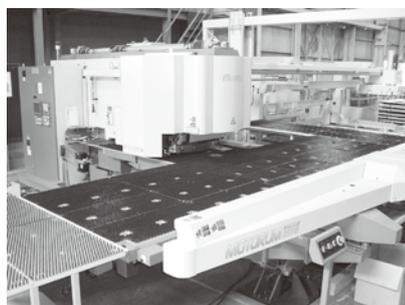
Sheet metal automatic machining system (Turret punch press, laser MFP)
